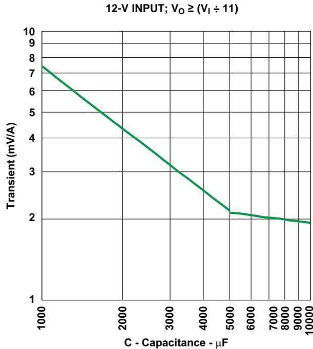
Figure 16. ( $V_O \geq V_I \div 11$ ) Capacitor Type B
