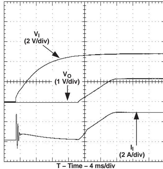
Figure 26. Power-Up Waveform
