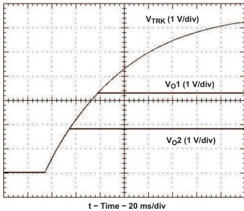
Figure 32. Simultaneous Power Up With Auto-Track Control
